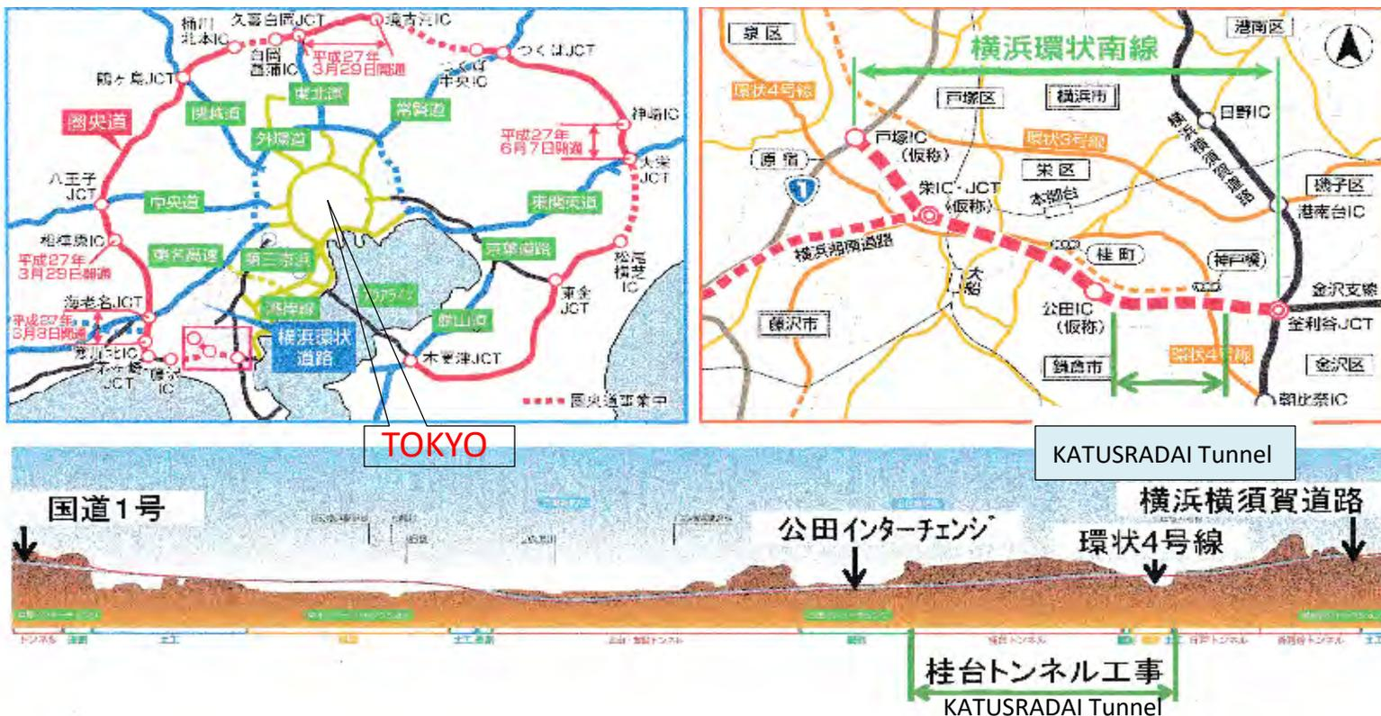
Total length: 1,7km Shield tunneling method
